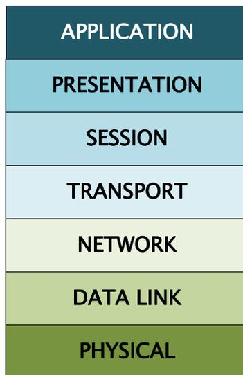
Fig. 1. OSI communications reference model
