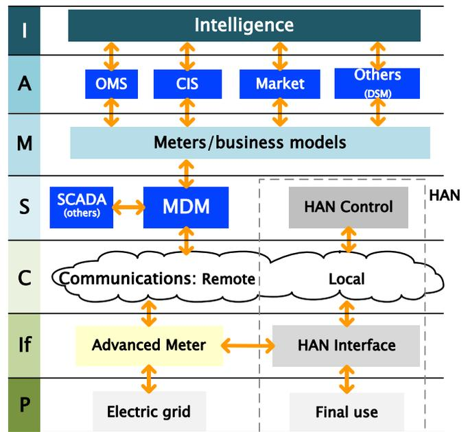
Fig. 5. Smart Grid Reference Model applied to AMI
