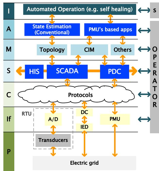
Fig. 4. SCADA/EMS System Model
