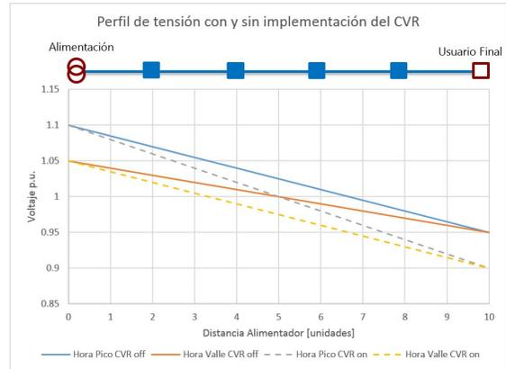
Fig. 2. Hypothetical voltage profile of a traditional feeder
