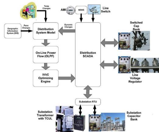
Fig. 4. DMS model based VVC (details of IVVC control components [9])
