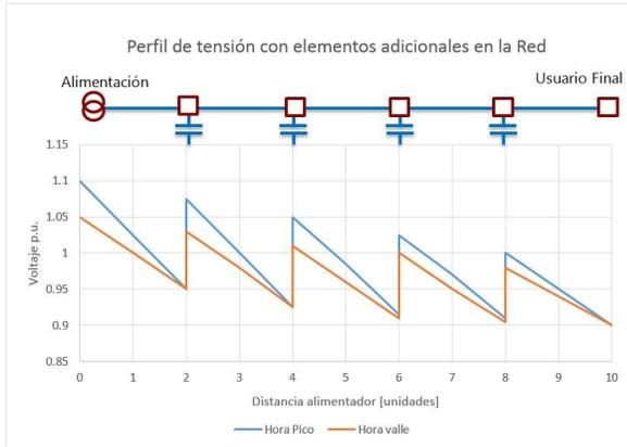
Fig. 3. Hypothetical voltage profile of a feeder with capacitor Banks
